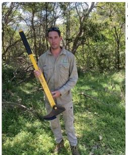
invested in some tree poppers. **Left:** Supervisor Sylvain gets ready for work. **Below:** Heavy metal jaws clamp onto the base of the stem, then the heel resting on the ground permits the whole plant to be levered out of the ground, roots and all. A very efficient way to remove Ochna.
